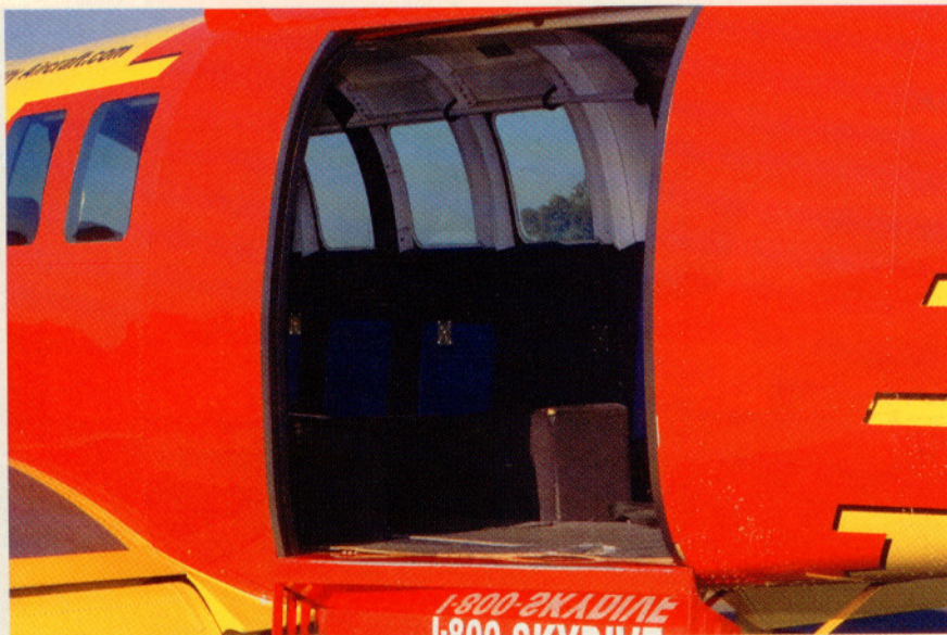
The PAC 750XL cabin door measures 50 inches wide (above). The simple panel features analog instruments (right).
